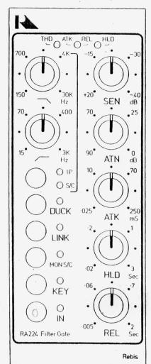
SEN: Adjusts the level at which the gate opens. (-40 to +20dBm)
